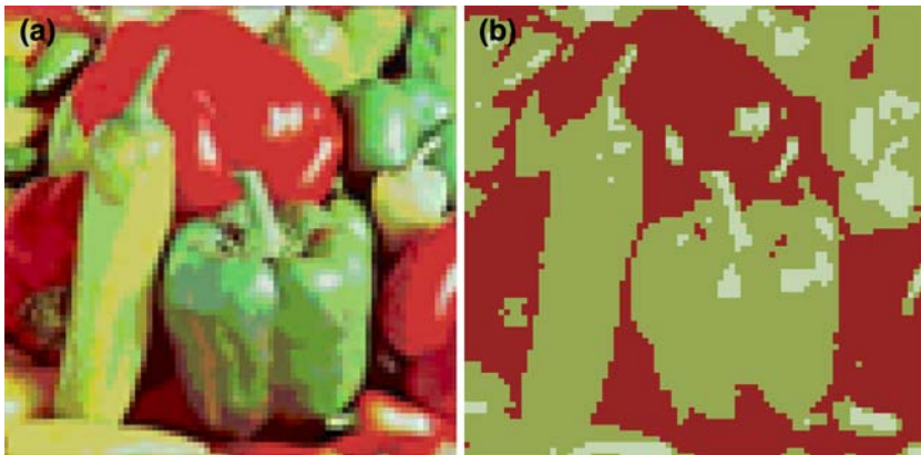
Figure 8. The segmentation result on the color image of peppers: (a) The original color image of peppers; (b) The segmented image of peppers via the adaptive gradient learning algorithm.
